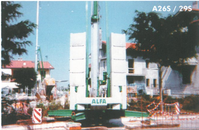
ZAVORRA MOBILE IN BLOCCHI DA KG. 1000/1250 ADDITIONAL BALLAST - BLOCK OF KG. 1000/1250
